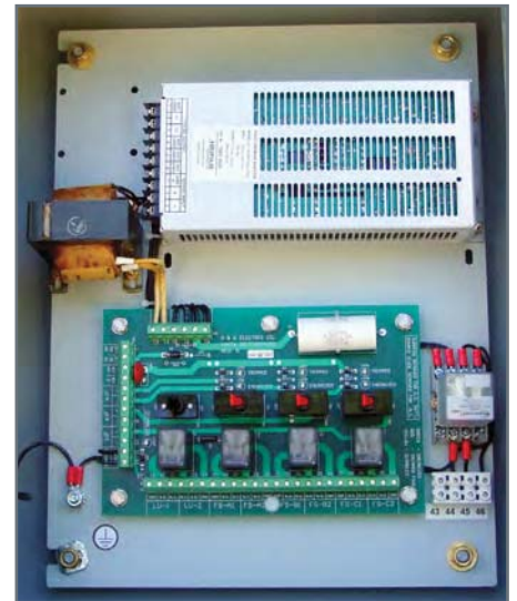
▲ Field test unit and redundant sensing and firing logic.
